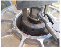
12) Be certain to properly align the "MASTER" spline for the spring retainer cap when re-installing.
