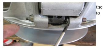
6)Install new primary spring into the clutch and re-install the cover onto the drive clutch (primary motor clutch). **Note: alignment marks.**
